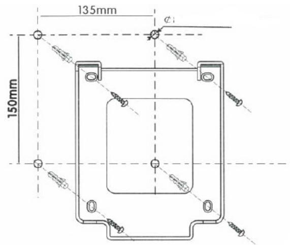
The mounting plate has a hook that the machine will hang onto. Place the machine above it and allow it to slot onto the hook.
