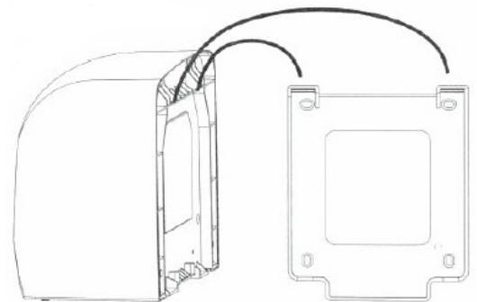
Screw the 'anti-theft' screws into the holes to fix the machine to the mounting plate.
