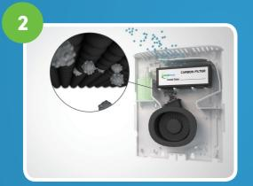
The air is then passed through the carbon filter which traps malodours, bacteria and VOCs.
