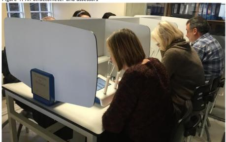
Figure 1: An olfactometer and assessors
