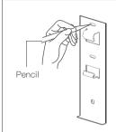
1.Attach mounting plate to the wall, 2.Use a drill to bore three holes use pencil to mark the position of (\$\phi6\$) according to the marks, put plastic nail — heads in the wall, installation three holes.
